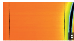
c. Resistivity map of multi-crystalline Si brick
